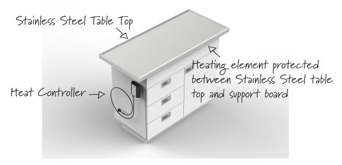
The Mark III LS Table with Heat is designed with Shor-Line's state of the art warming system. The stainless steel table top measures 20" wide and 44.5" long with raised edges to prevent fluid runoff. The table provides plenty of storage space with 3 drawers and 1 door. The warming system is operated by a control box which is mounted on the top front left side of the cabinet.
