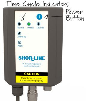
temperature protection of 97° F (36.11° C). If for any reason the table reaches a temperature of 97° F (36.11° C), the heater will be disabled, the alert light will illuminate red and flash continuously and a triple beep will occur. This condition will remain until the table lowers in temperature or the unit is turned off by pressing the Power Button.
