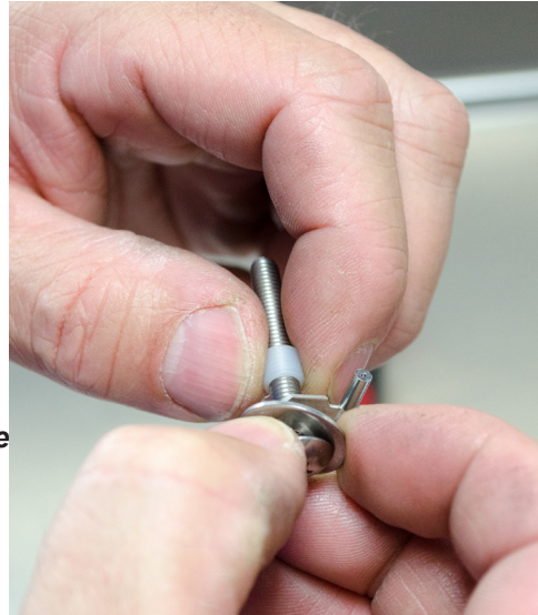
FIGURE 2.33 - Quick Release Assembly
