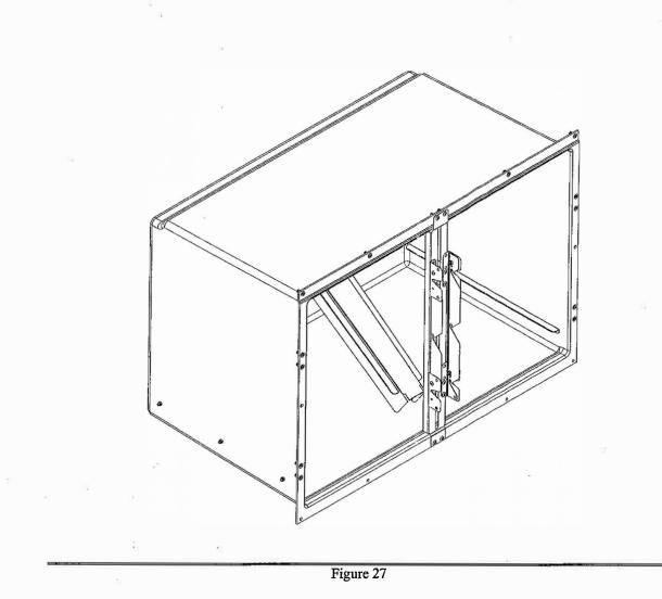
Insert floor spacer assembly as shown in Figure 27, and see next step.
